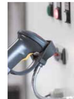
Simple and secure data handling with integrated USB and LAN interface. Recipes can be called up simply and safely with the barcode reader. Integration of the machines in internal company structures with remote access and online machine access is possible. OPC-UA is available as a universal communication interface on all our machines.
