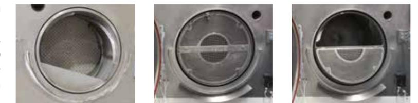
The basket can be swapped and a variety of basket perforations are therefore available. Tailored exactly to your requirements according to the moulded part sizes. Loading occurs manually via the manually operated exterior door. The basket is automatically emptied by means of the integrated roller rails.
