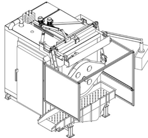
**AWS 40 WITH FULLY AUTOMATED LOADING DOOR AND LOADING**
